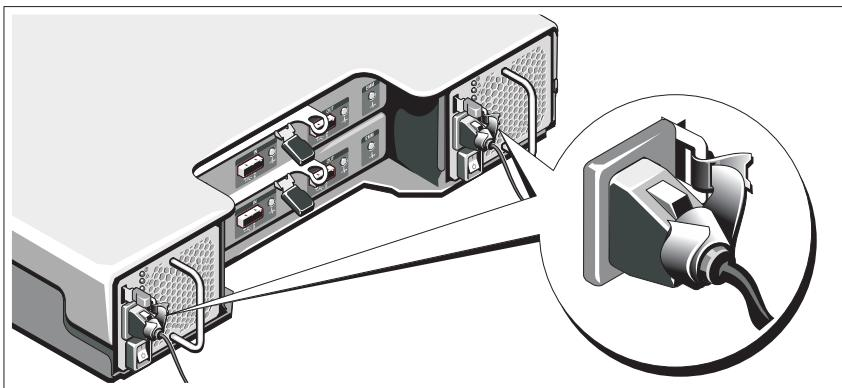
Bend the system power cable(s) as shown in the illustration and secure the cable(s) firmly to the bracket using the provided strap.
